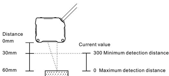
For example, when using the defaults with the setting value at 150, the comparator output turns on when the current value is 150 or greater and turns off when it is less than 148. (The hysteresis value is set to 2 by default, and if the hysteresis value is set to 0, the current value is closed when the value is less than 150).
