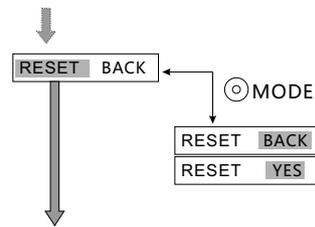
long press [MODE] (>3s) to complete the setting and return to the detection state.
